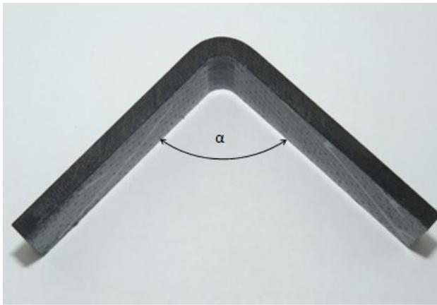
Fig. 1: Curved beam strength sample
