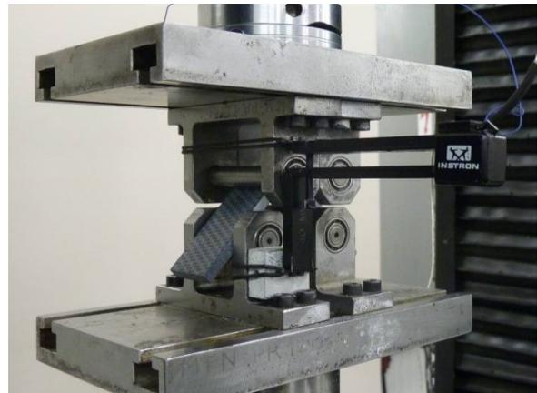
Fig. 2: Curved beam strength test
