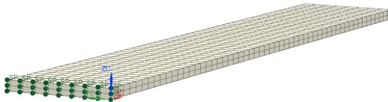
Fig. 5: FE model of the beam.
