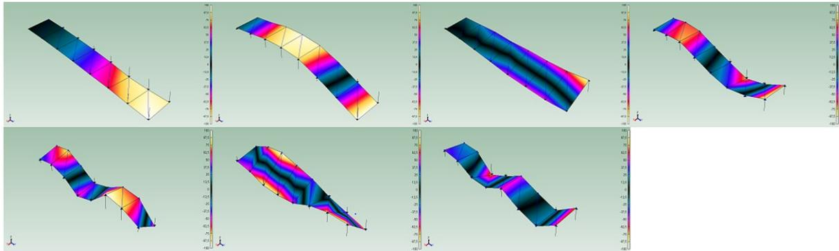
Fig. 4: Mode shapes of the beam.
