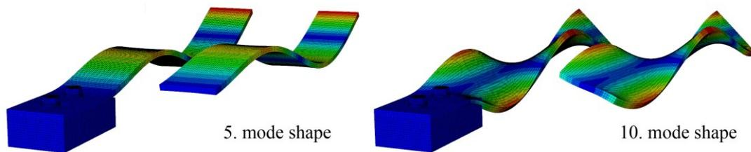
Fig. 2: Selected mode shapes of compared models.
