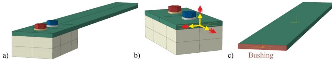
Fig. 1: a) The complete initial FEM model, b) Part of the model used to obtain stiffness parameters, c) The equivalent model with bushing connector.
