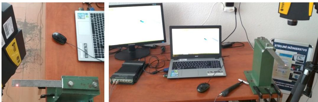
Fig. 3: Experimental modal analysis of the beam.
