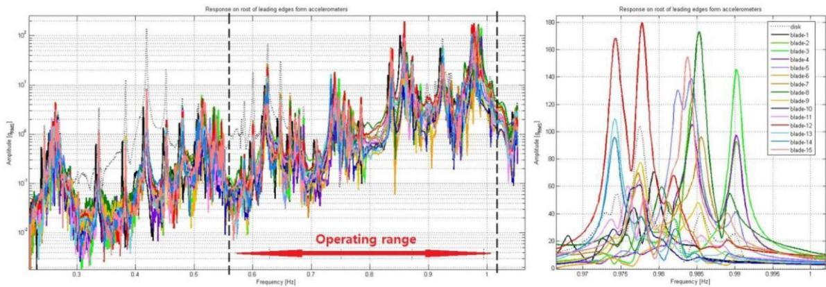
Fig. 7: Spectra measured with accelerometers at the root of leading edges
