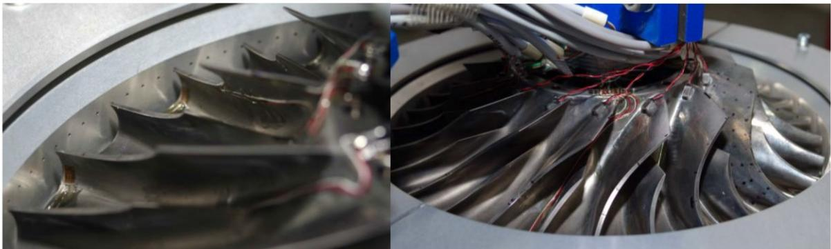
Fig. 5: Placement of the strain gauges on the trailing edge of the impeller blades and accelerometers on root of leading edges
