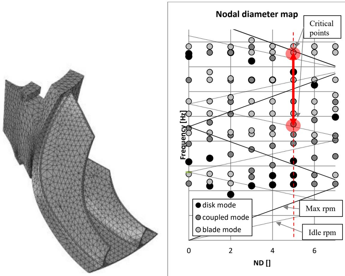
Fig. 2: a) FE model segment of centrifugal compressor and b) SAFE diagram
