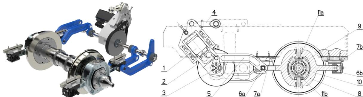
Fig. 7: Wheelset steering mechanism
