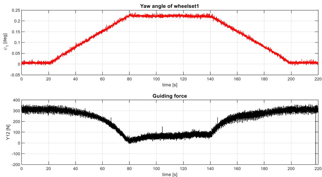
Fig. 10: Measured data – active wheelset steering test
