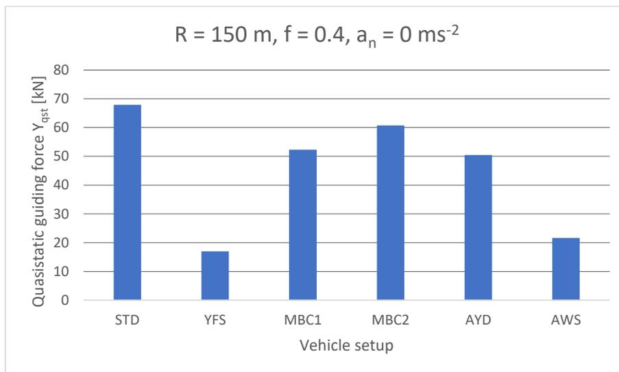
Fig. 3: Quasistatic guiding force  $Y_{qst}$  acting on outer wheel of the 1<sup>st</sup> wheelset in curve with radius  $R = 150$  m for various vehicle configurations
