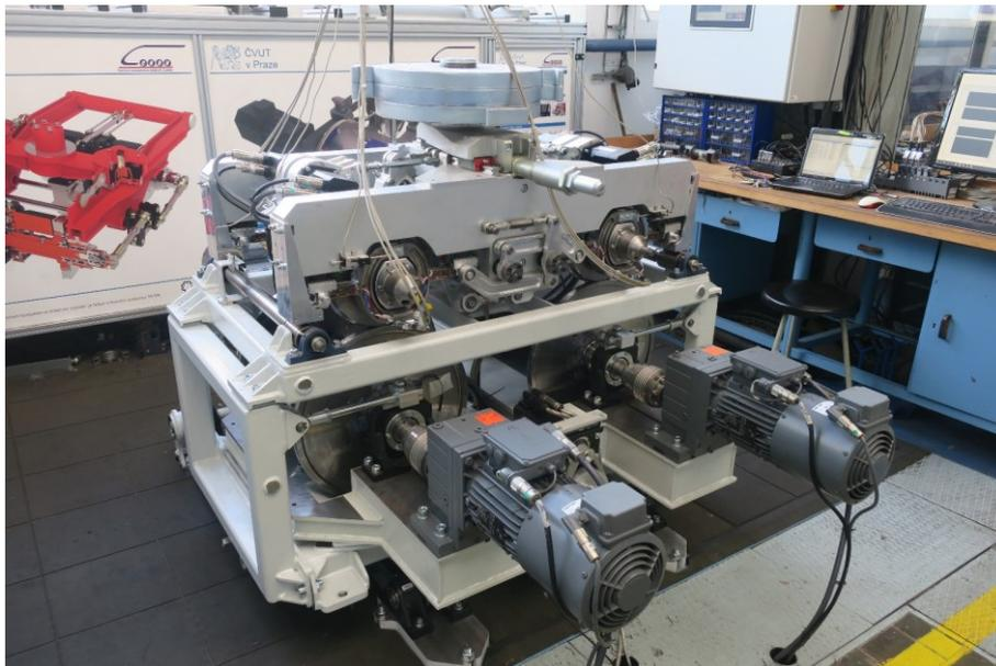
Fig. 4: Scaled roller rig of the Czech Technical University
