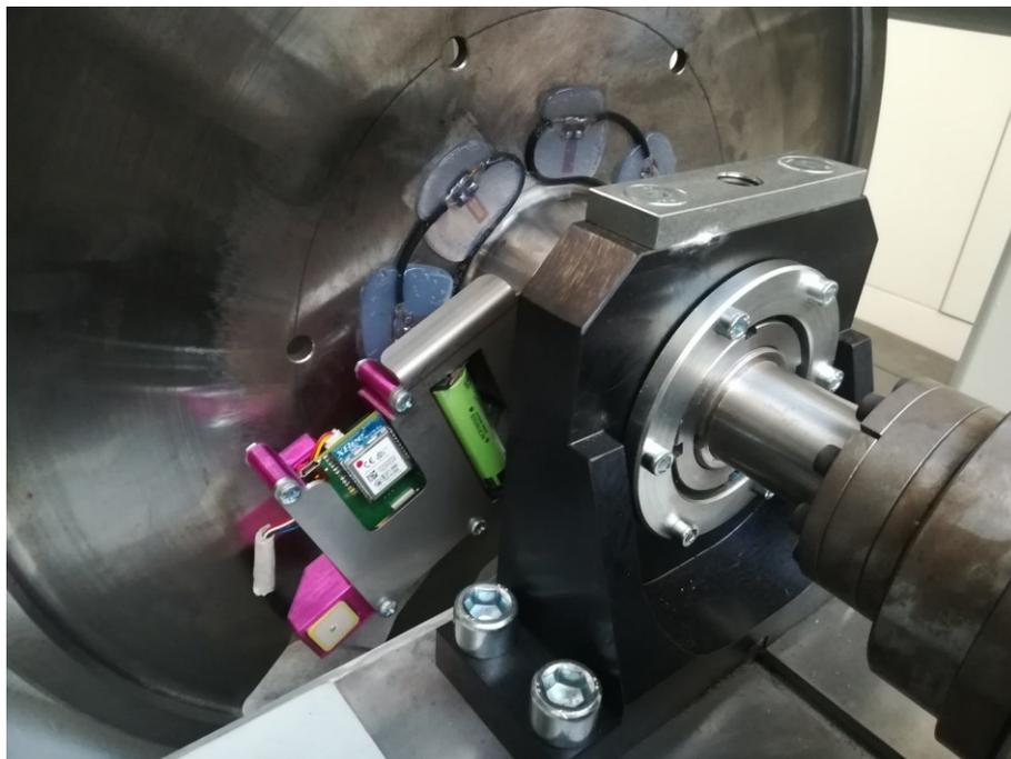
Fig. 6: Strain gauge instrumented roller with wireless transmitter module
