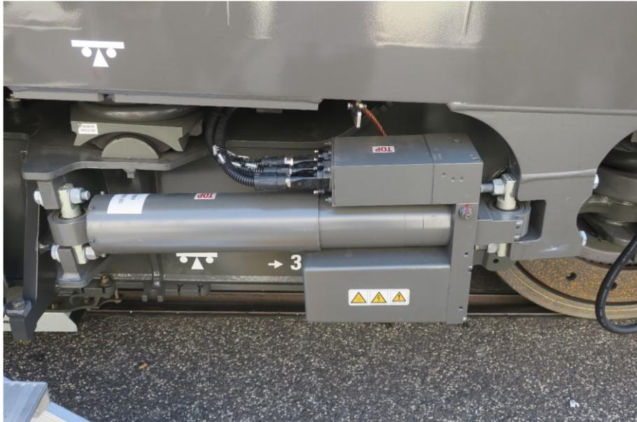
Fig. 1: Active yaw damper on Siemens Vectron MS locomotive for ÖBB, Innotrans fair 2018 (photo author)
