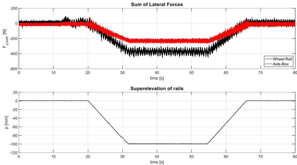
Fig. 9: Measured data – vehicle run in a canted straight track
