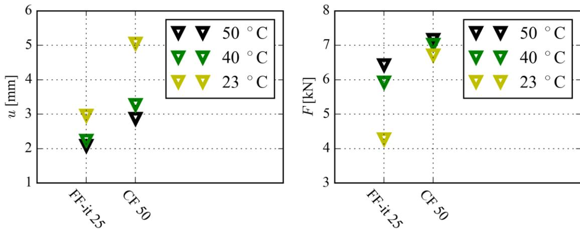
Fig. 4: The temperature influence: a) Minimal height of the sample during the drop test, b) maximal transmitted force
