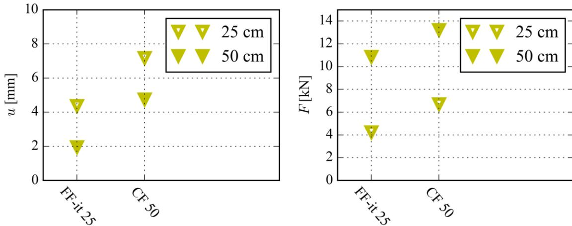
Fig. 3: a) Minimal height of the sample during the drop test, b) maximal transmitted force
