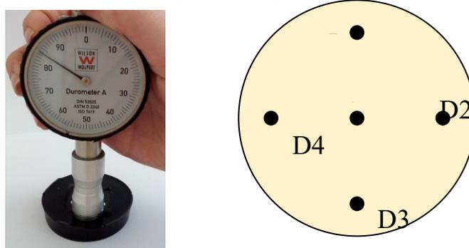
Fig. 1: a) Verification of Shore A value, b) measured positions
