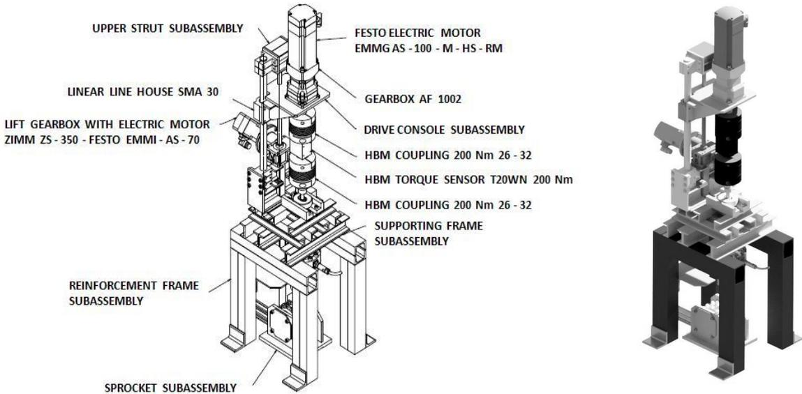
Fig. 11: Testing equipment for complex analysis of screw fasteners [Author]
