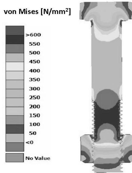
Fig. 8: Examples of FEM analysis of the prestressed bolted connection for bolt of size *M16*, strength class *12.9*, loaded by external static axial force of *40 kN*; equivalent stresses in the bolted connection for bolt of size *M16*, strength class *12.9*, loaded by external static axial force of *40 kN* [Author]
