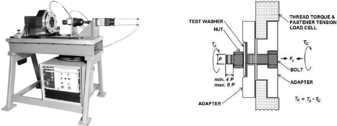
Fig. 10: Laboratory fastener test machine, typical, (on the left side). Torque-tension research head, (on the right side) [5]
