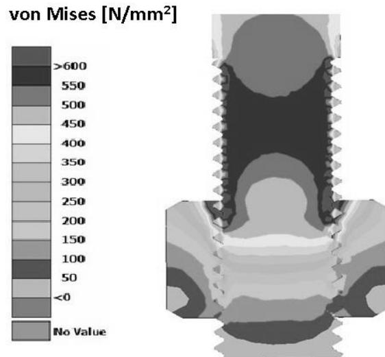
Fig. 9: Examples of FEM analysis of the prestressed bolted connection for bolt of size *M16*, strength class *12.9*, loaded by external static axial force of *40 kN* (detailed view); equivalent stresses in the bolt of size *M16*, strength class *12.9*, loaded by external static axial force of *40 kN* [Author]
