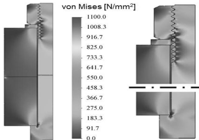
Fig. 5: Examples of FEM analysis of the prestressed bolted connection for bolt of size *M20*, strength class *12.9*, loaded by external static axial force of *55 kN* [4]
