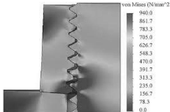
Fig. 6: Examples of FEM analysis of the prestressed bolted connection for bolt of size *M24*, strength class *10.9*, loaded only by assembly static preload of *312 kN* [4]
