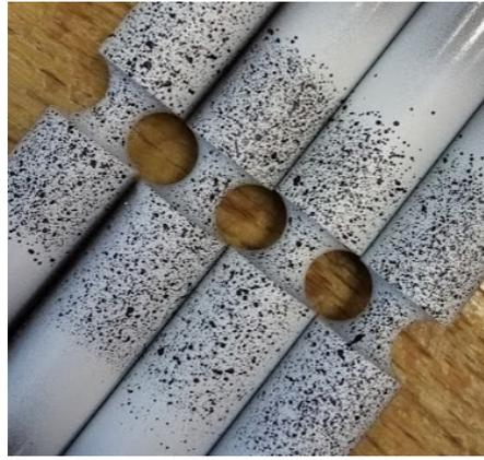
Fig. 3: Representative pattern for DIC measurement
