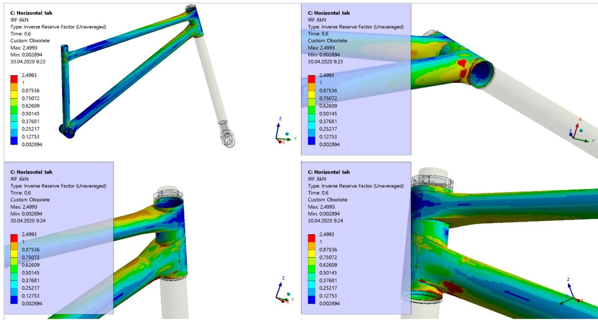
Fig. 14: IRF factor from Ansys analysis for 6 kN tension force
