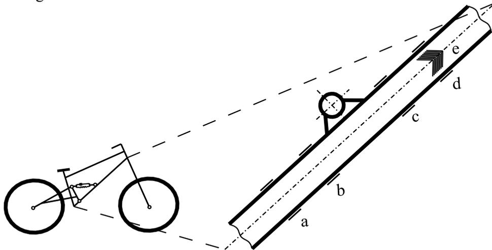
Fig. 2: Scheme of the frame and the positions of the strain gauges on the down tube
