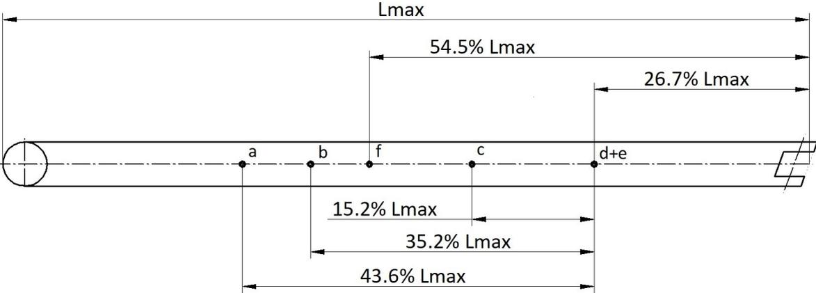
Fig. 4: Distances of positions of SGs and shock absorber on down tube
