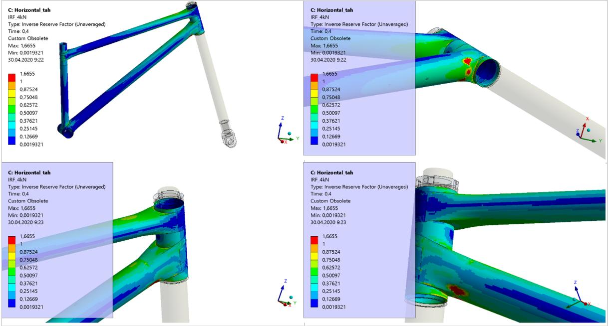
Fig. 13: IRF factor from Ansys analysis for 4 kN tension force
