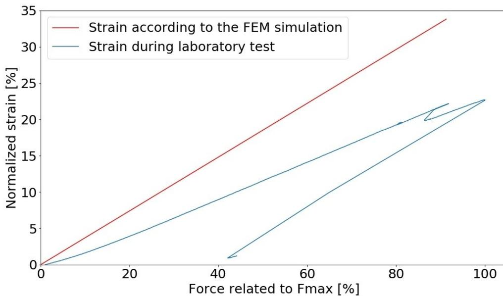
Fig. 16: Comparison of FEM analysis and experimentally measured dependence between force and strain
