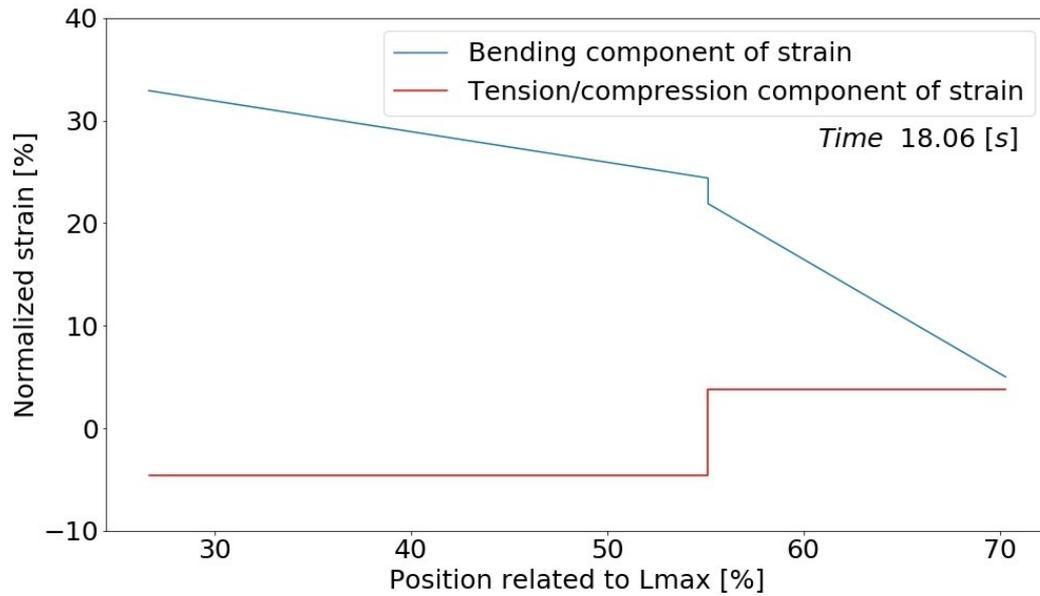
Fig. 8: Distribution of bending and tension/compression component of strain along DT during landing part
