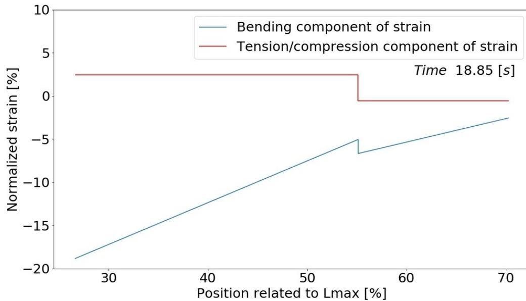
Fig. 9: Distribution of bending and tension/compression component of strain along DT during routine driving
