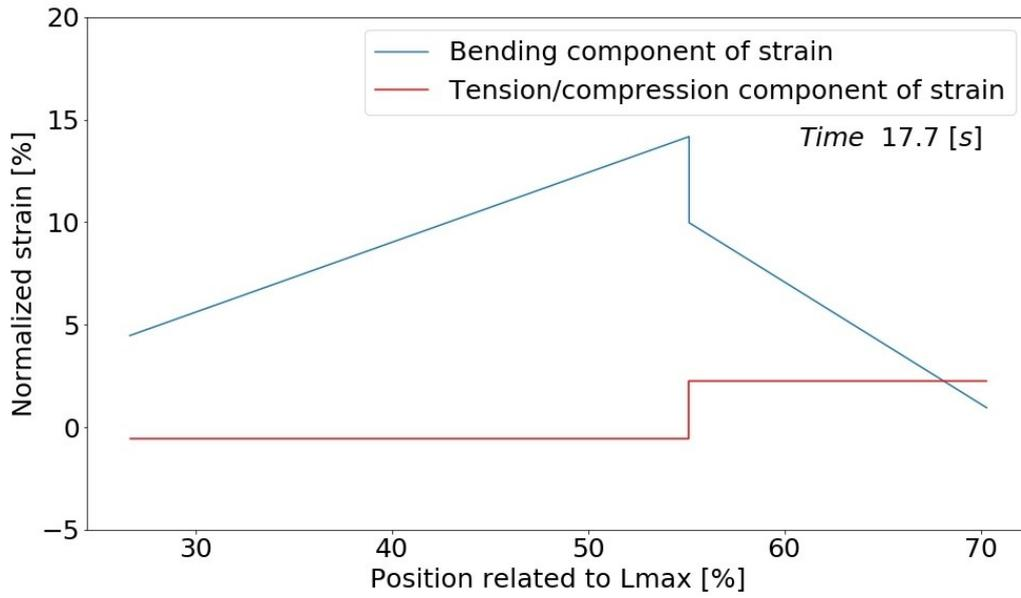
Fig. 6: Distribution of bending and tension/compression component of strain along DT during take-off
