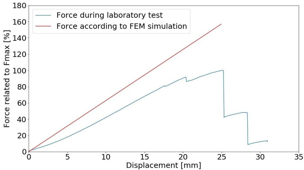
Fig. 15: Comparison of FEM analysis and experimentally measured dependence between force and displacement
