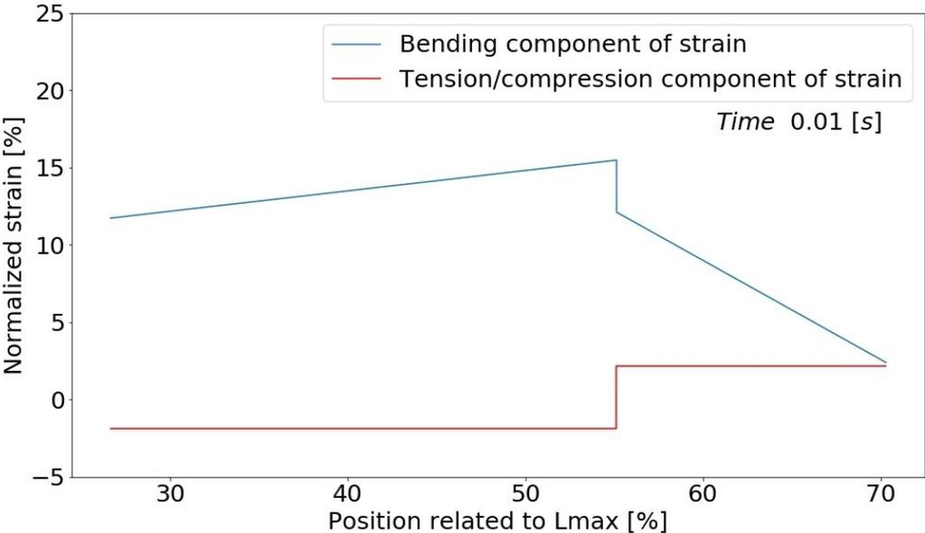
Fig. 5: Distribution of bending and tension/compression component of strain along DT in static state mode with sitting rider
