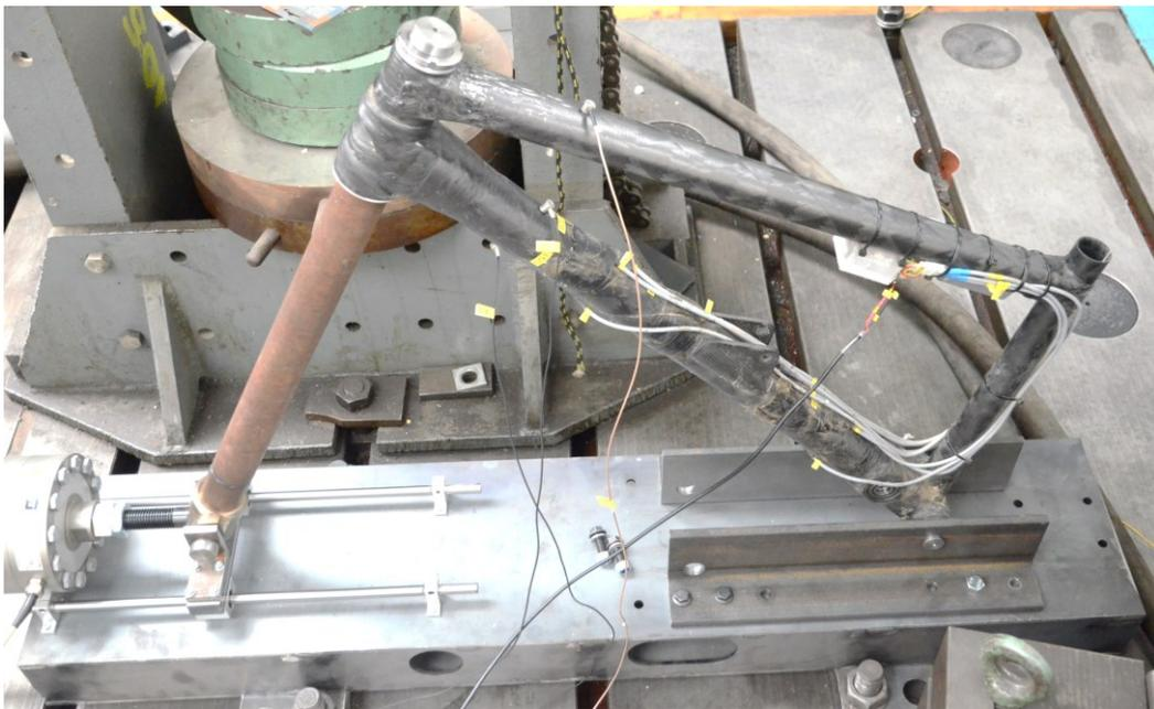
Fig. 10: Laboratory test stand for quasi-static and fatigue load cases
