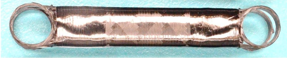
Fig. 1: CFRP filament wound tubes with ILT joint
