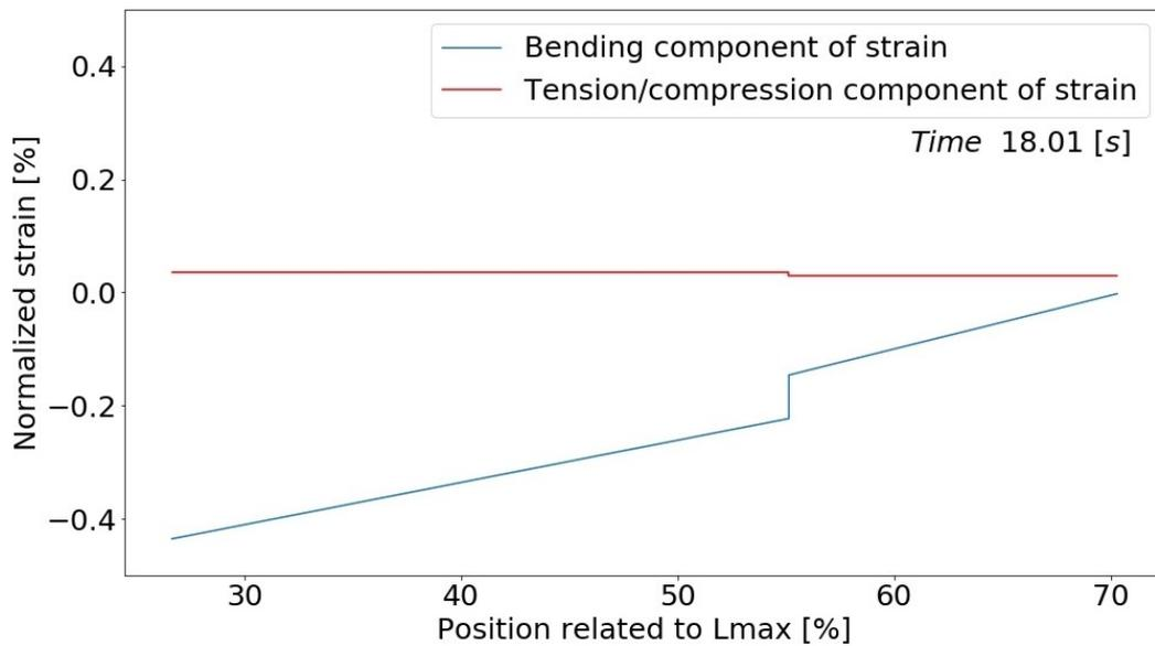
Fig. 7: Distribution of bending and tension/compression component of strain along DT during fly
