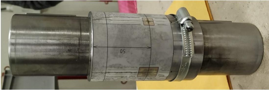
Fig. 5: Applied application foil with strain gauges on the input shaft (Location 1 in Fig. 4)
