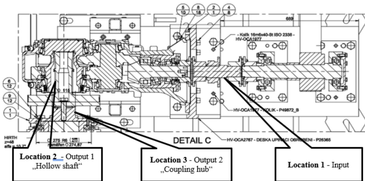
Fig. 4: Drawing with determination of places for application of strain gauges
