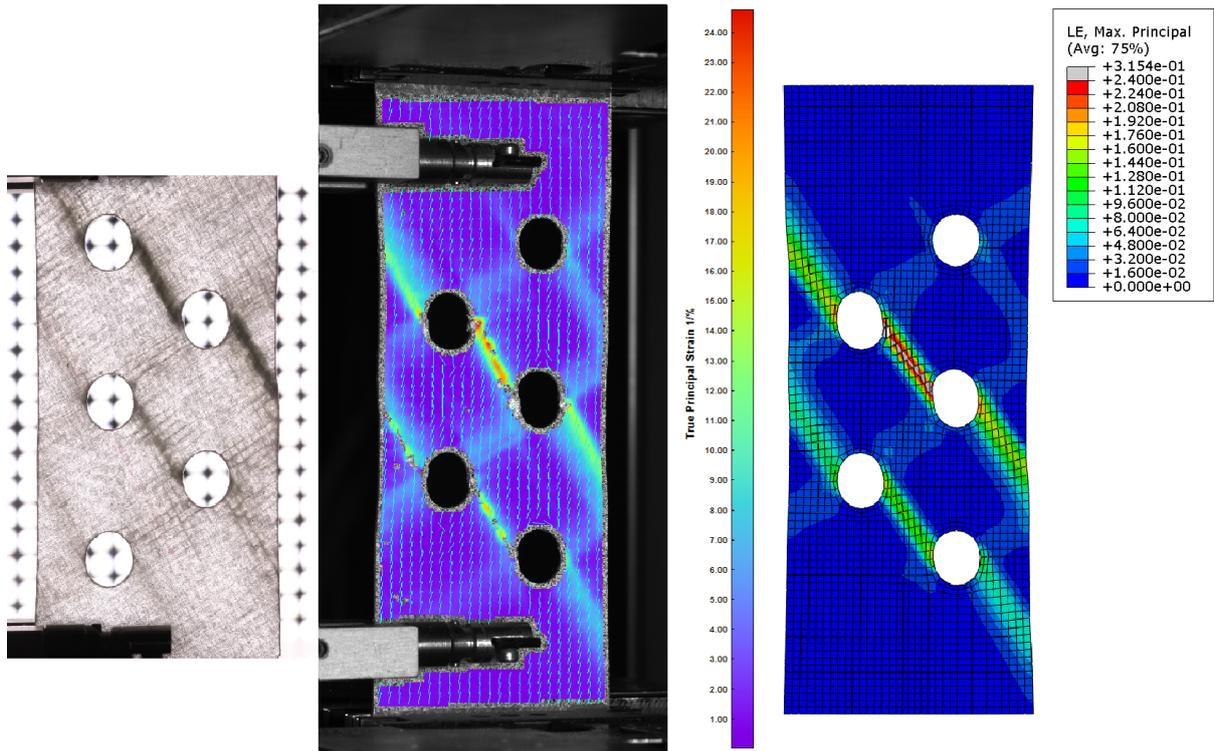
Fig. 10: Visual comparison of results for specimen TH-30 and displacement  $u = 3.0$  mm: the backlight illuminated specimen (left), the maximum true principal strain as resolved by the DIC system (center) and as computed by the numerical simulation (right)
