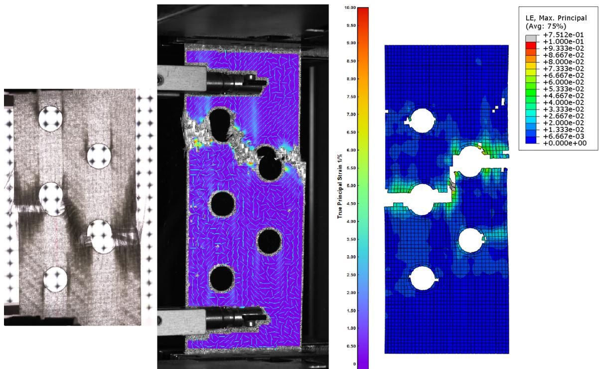
Fig. 7: Visual comparison of results for specimen TH-0 at the end of loading: the backlight illuminated specimen (left), the maximum true principal strain as resolved by the DIC system (center) and as computed by the numerical simulation (right)
