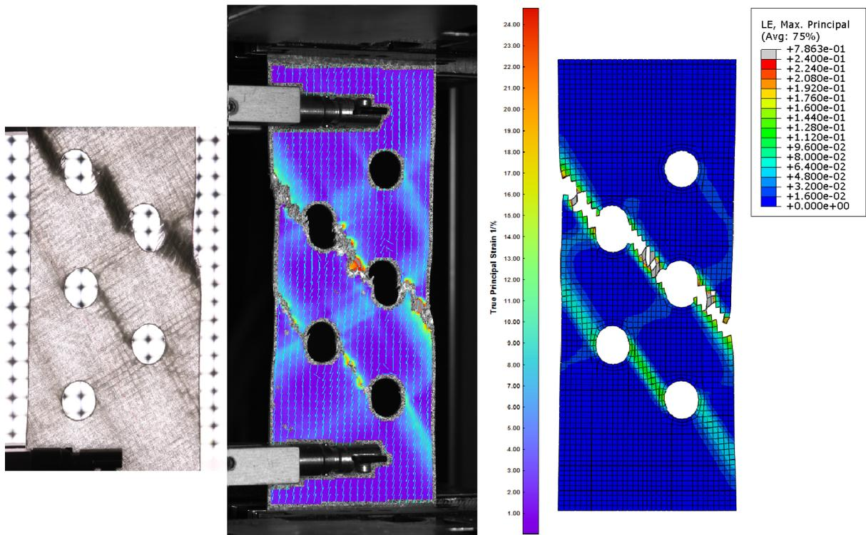
Fig. 11: Visual comparison of results for specimen TH-30 and displacement  $u = 4.0$  mm: the backlight illuminated specimen (left), the maximum true principal strain as resolved by the DIC system (center) and as computed by the numerical simulation (right)
