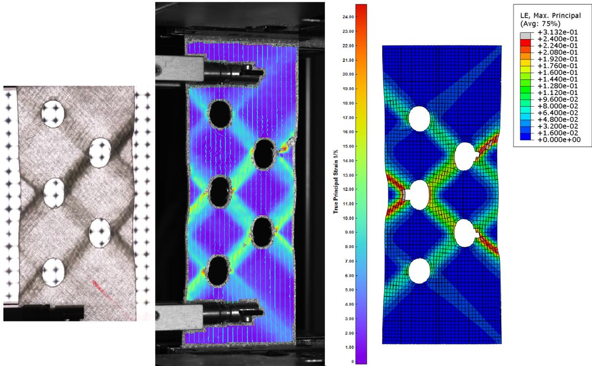
Fig. 12: Visual comparison of results for specimen TH-45 and displacement  $u = 5.0$  mm: the backlight illuminated specimen (left), the maximum true principal strain as resolved by the DIC system (center) and as computed by the numerical simulation (right)
