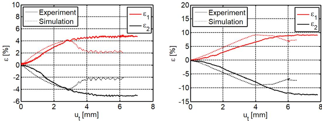
Fig. 5: Relation between the true principal strains (maximum  $\varepsilon_1$  and minimum  $\varepsilon_2$  true principal strain) and the total displacement for specimens TH-30 (left) and TH-45 (right), comparison between experimental and computational results at point no. 2
