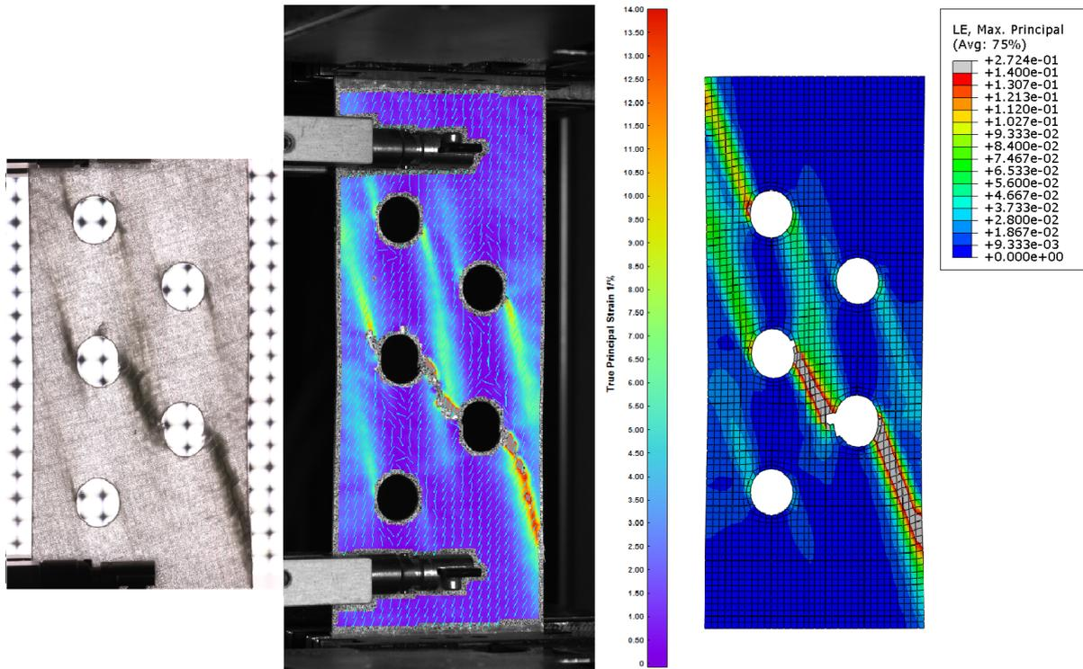
Fig. 8: Visual comparison of results for specimen TH-15 and displacement  $u = 2.0$  mm: the backlight illuminated specimen (left), the maximum true principal strain as resolved by the DIC system (center) and as computed by the numerical simulation (right)
