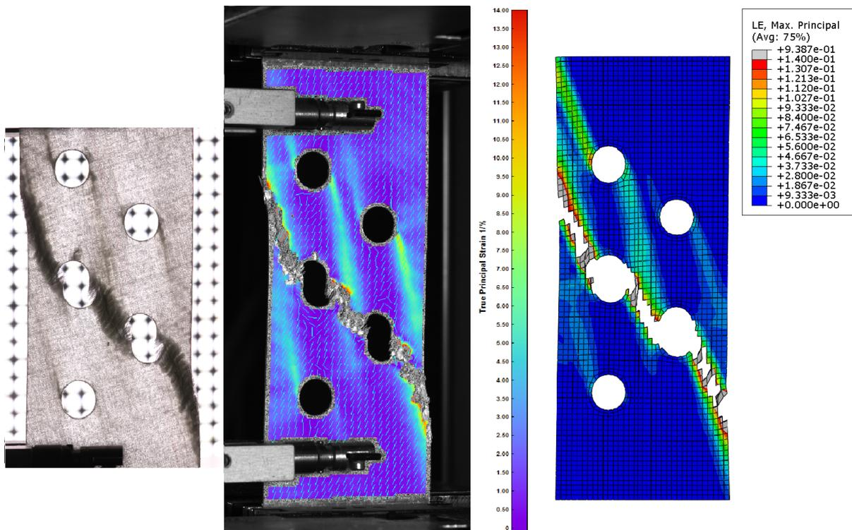
Fig. 9: Visual comparison of results for specimen TH-15 and displacement  $u = 4.0$  mm: the backlight illuminated specimen (left), the maximum true principal strain as resolved by the DIC system (center) and as computed by the numerical simulation (right)
