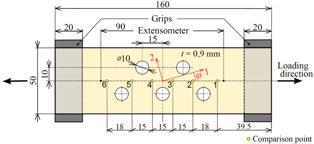
Fig. 1: The perforated specimen geometry and the experimental setup
