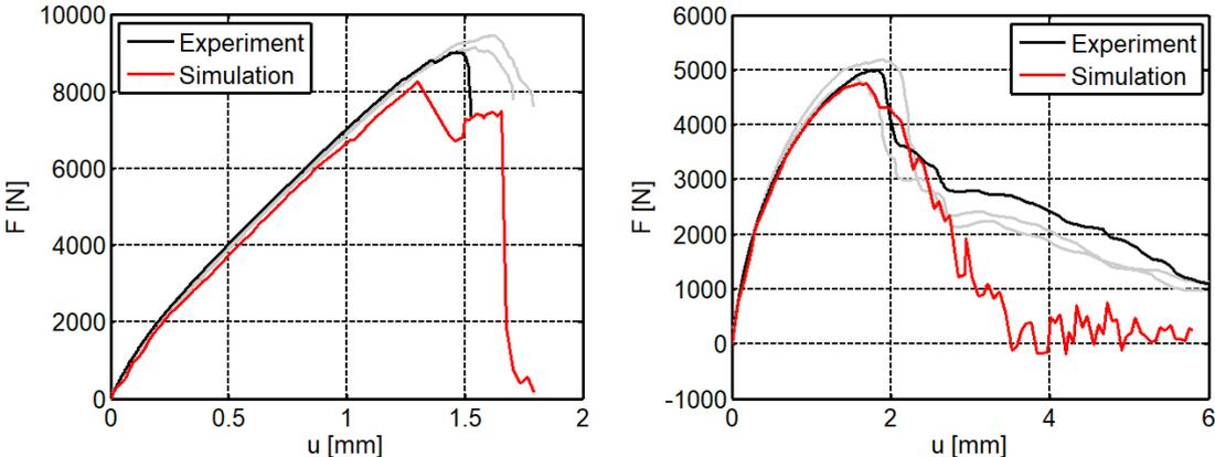
Fig. 2: Force-displacement diagram comparison between experimental and numerical results for specimens TH-0 (left) and TH-15 (right)
