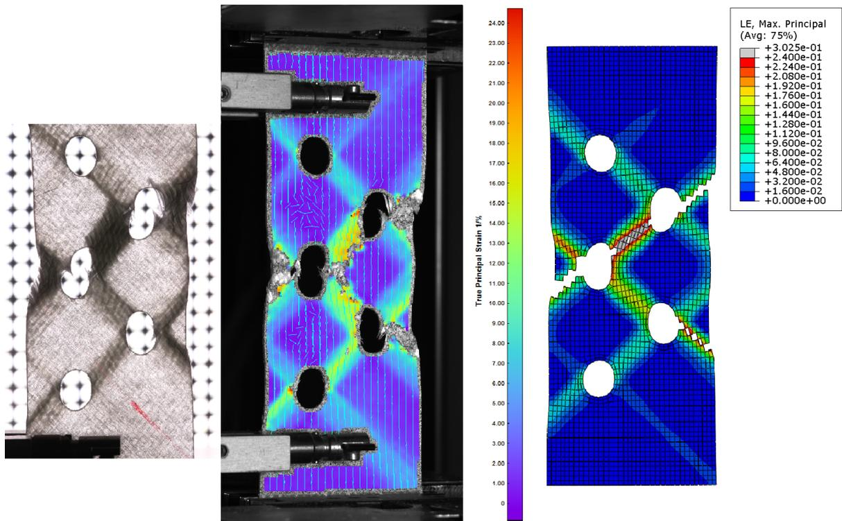
Fig. 13: Visual comparison of results for specimen TH-45 and displacement  $u = 7.0$  mm: the backlight illuminated specimen (left), the maximum true principal strain as resolved by the DIC system (center) and as computed by the numerical simulation (right)
