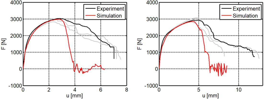
Fig. 3: Force-displacement diagram comparison between experimental and numerical results for specimens TH-30 (left) and TH-45 (right)
