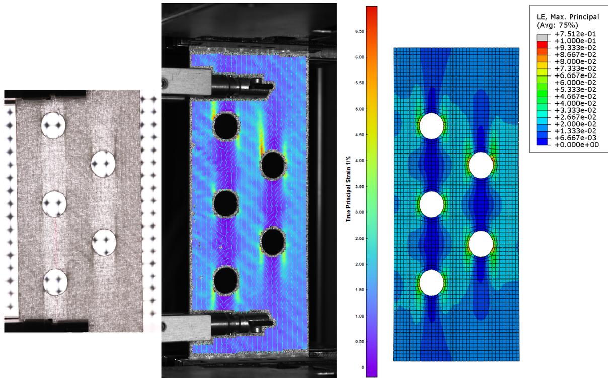
Fig. 6: Visual comparison of results for specimen TH-0 and loading force  $F = 8000 \text{ N}$  ( $u = 1.2 \text{ mm}$ ): the backlight illuminated specimen (left), the maximum true principal strain as resolved by the DIC system (center) and as computed by the numerical simulation (right)
