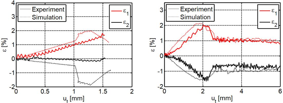
Fig. 4: Relation between the true principal strains (maximum  $\epsilon_1$  and minimum  $\epsilon_2$  true principal strain) and the total displacement for specimens TH-0 (left) and TH-15 (right), comparison between experimental and computational results at point no. 2
