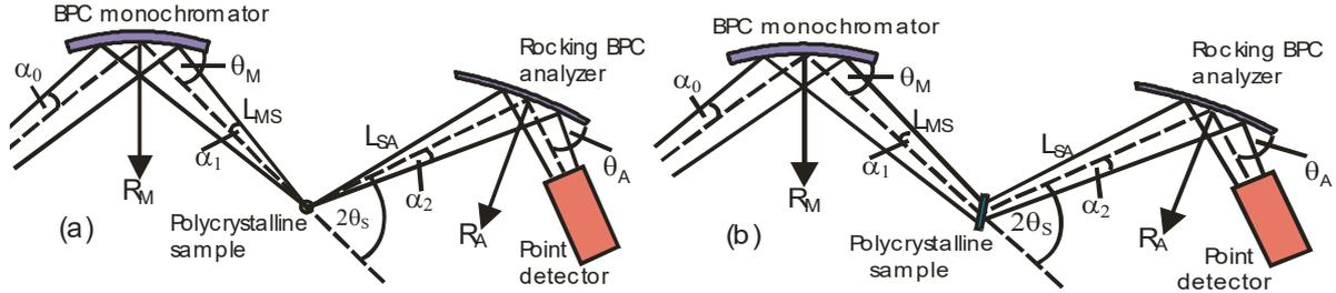
Fig. 2: Scheme of the three axis diffractometer performances employing BPC monochromator and analyzer operating with bar samples in vertical – (a) and/or in horizontal position – (b) with a point detector ( $R_M$ ,  $R_A$  - radii of curvature,  $\theta_M$ ,  $\theta_A$  - Bragg angles).
