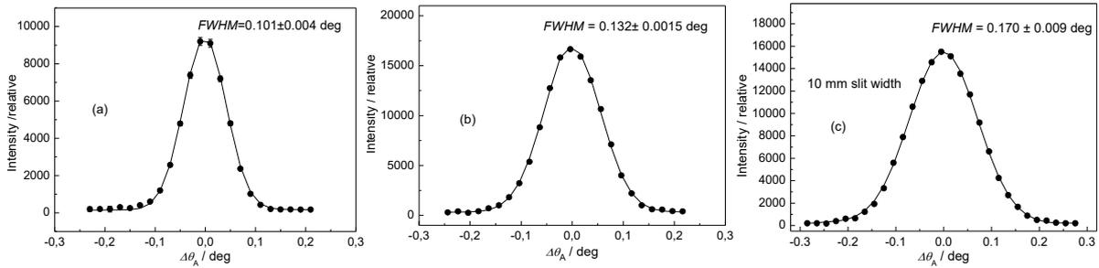
Fig. 3: Analyzer rocking curves for the virgin  $\alpha$ -Fe(110) samples of (a) -  $\phi=5.1 \text{ mm}$  and (b) -  $\phi=8 \text{ mm}$  situated in the vertical position and the sample of (c) -  $\phi=8 \text{ mm}$  in the horizontal position (see Fig. 2b).
