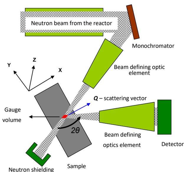
Fig. 1: Schematic drawing of the conventional strain scanner.
