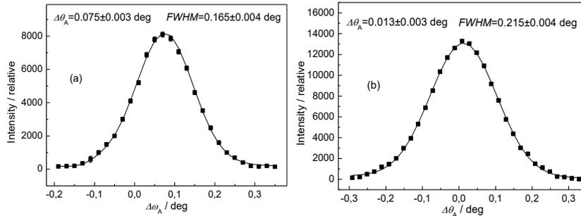
Fig. 5. Analyzer rocking curves for the deformed  $\alpha$ -Fe(110) steel wire installed in the vertical – (a) and horizontal position – (b).
