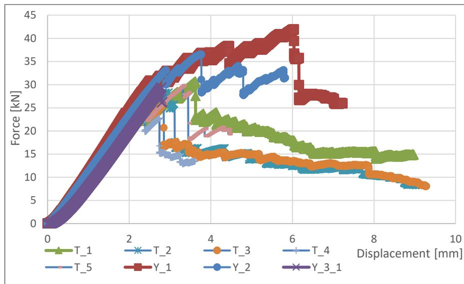
Fig. 1 Relationship between loading force and displacement for tested specimens
