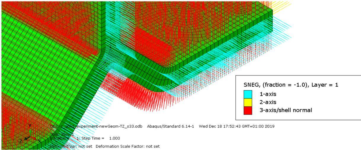
Fig. 3 Material orientation in the beam
