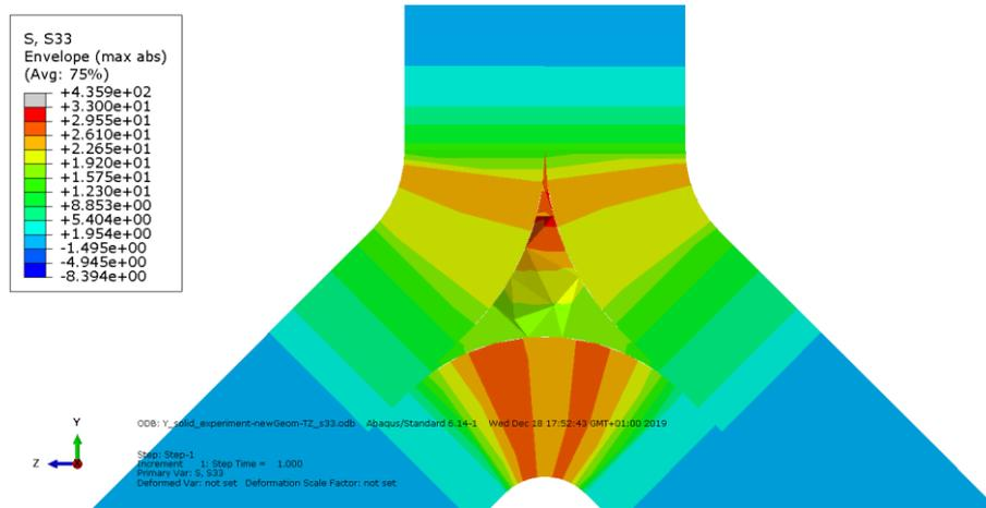
Fig. 6 S33 stress field in the failed area
