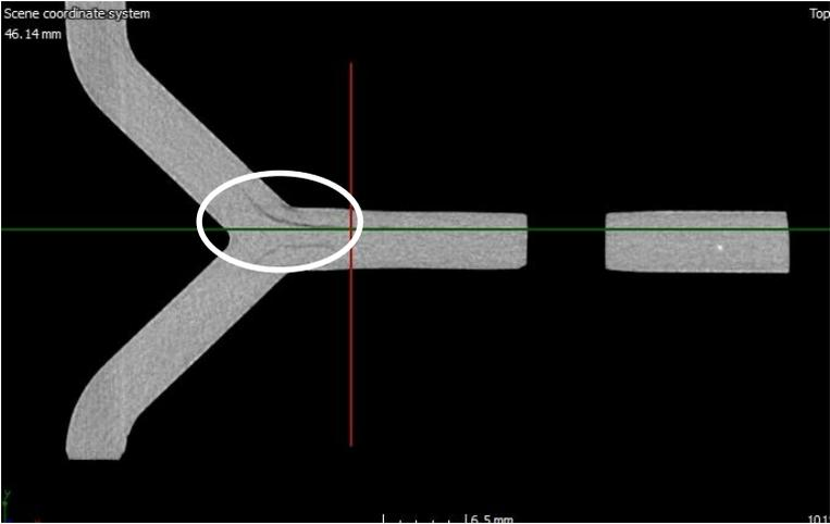
Fig. 2 Failure area evaluated from CT scan
