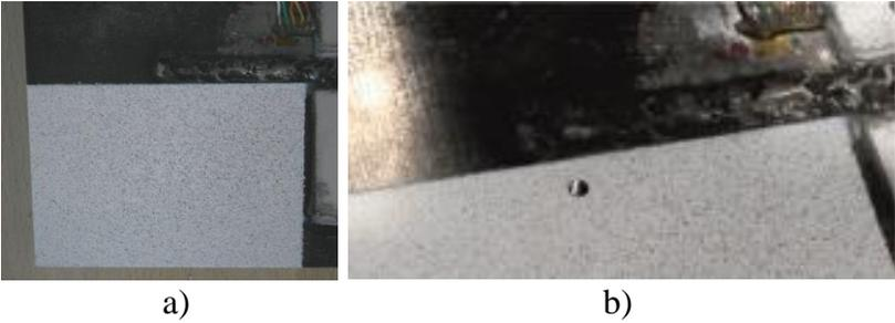
Fig. 15: Specimen with the applied stochastic pattern a) whole view, b) hole drilled near the weld joint
