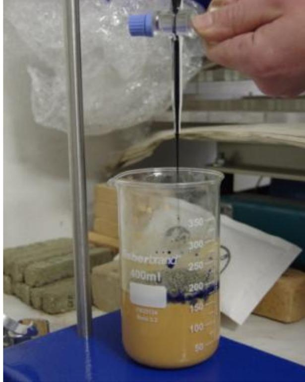
Fig. 1: Dye dosed into the earth sample
