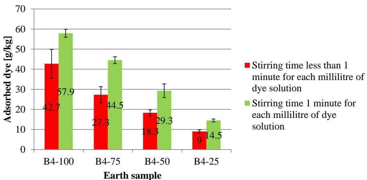
Fig. 4: Amount of adsorbed dye by kaolinite clay (B4) before and after modification of methodology
