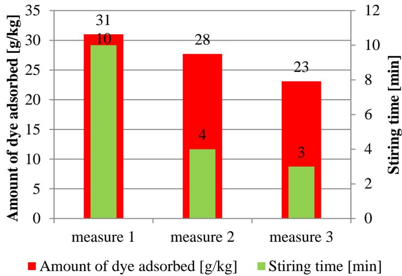
Fig. 3: Amount of adsorbed dye by kaolinite clay (sample B4-75: 11.25 g kaolinite clay, 3.75 g sand)
