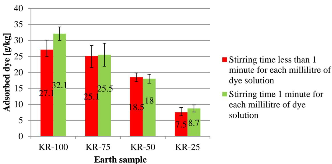
Fig. 5: Amount of adsorbed dye by illite-kaolinite clay (KR) before and after modification of methodology
