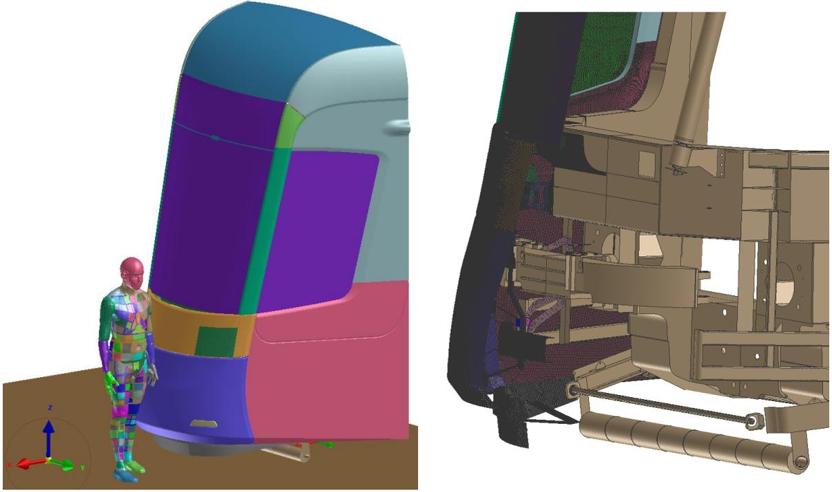
Fig. 2: Numerical model of the collision (left) and detail of tram FE structure (right)
