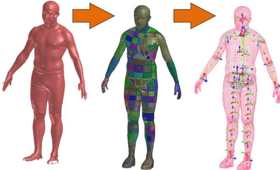
Fig. 1: VIRTHUMAN model CAD data, FE model and Multibody structure
