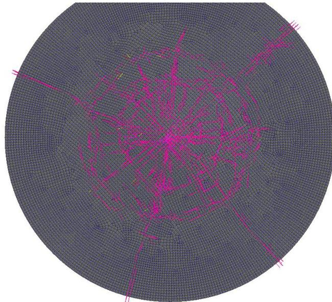
Fig. 4: The windshield glass with damage tensor directions
