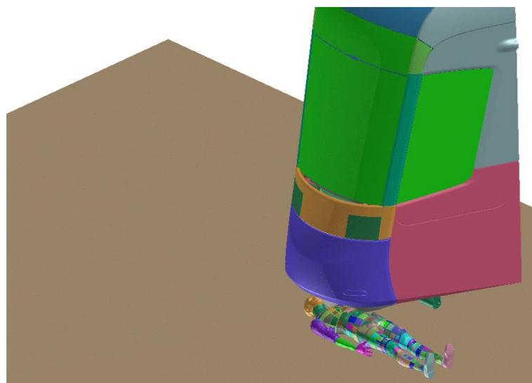
Fig. 9: The result of simulation of tram and laying pedestrian (90 ms)
