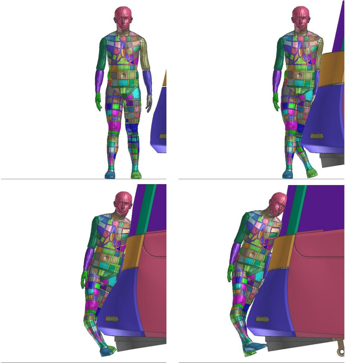
Fig. 7: The results of simulation (in time 0, 25, 50, 75 ms), where the head impacts the windshield
