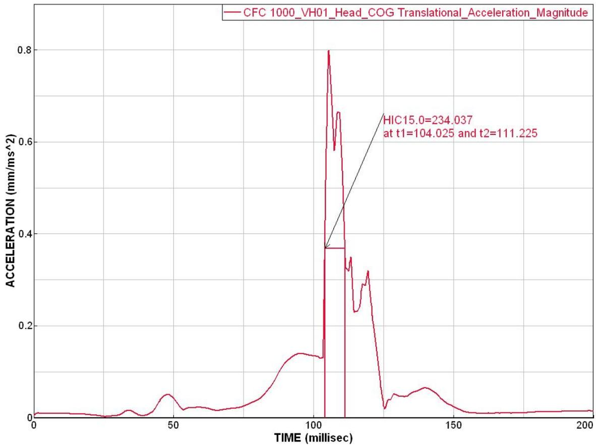
Fig. 8: The acceleration of the COG filtered by CFC1000 filter with HIC15 injury criterion assessment
