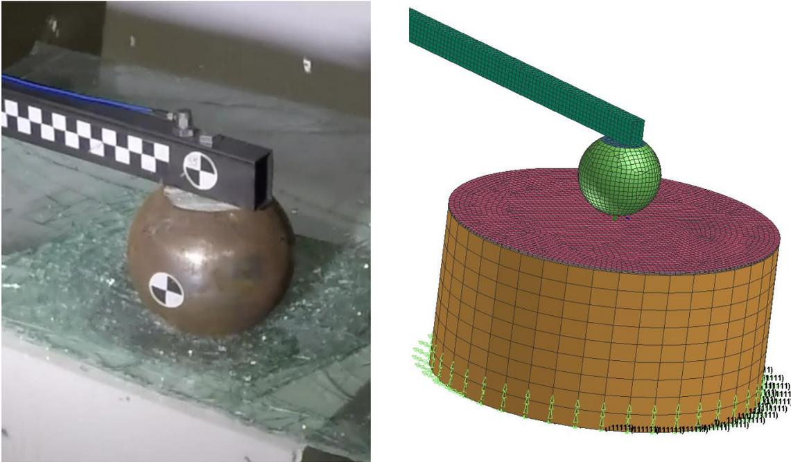
Fig. 3: Experimental test of windshield (left) and simulation for material validation (right)
