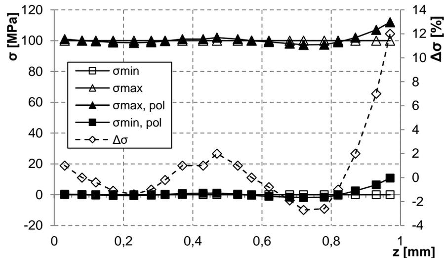
Fig. 1: Ideal stress profile for pure tension and distortion using polynomial interpolation
