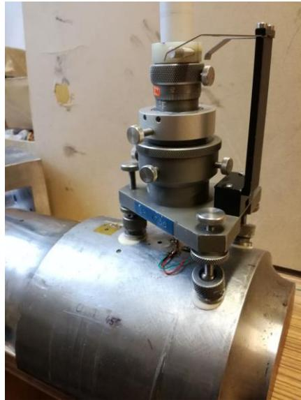
Fig. 3: Investigated half section of the axle and used drilling device Vishay RS-200
