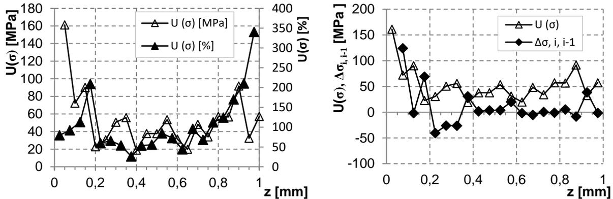
Fig. 5 Error analysis of real measurement (left absolute and relative values, right comparison of the uncertainty with the stress difference between two adjacent steps)
