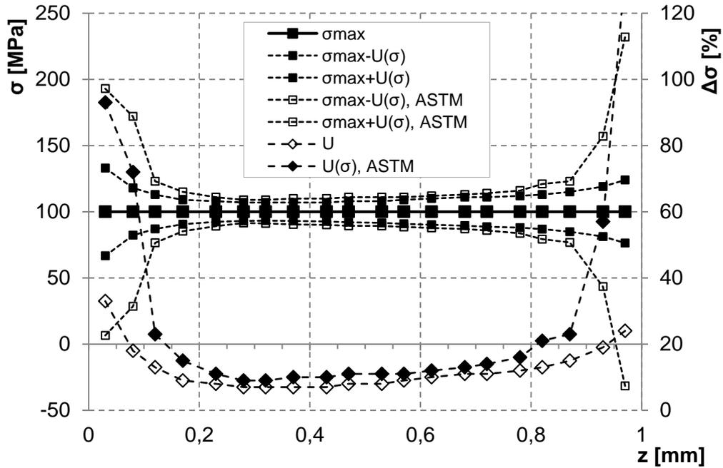
Fig. 2: Uncertainty tolerance limits for pre-set and critical ASTM input uncertainties
